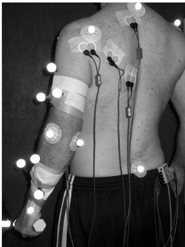
Figure 2. Photograph depicting reflective marker and electrode placement.
